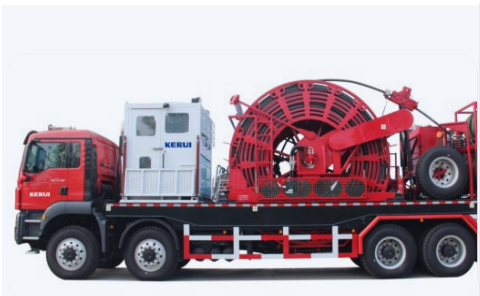
12 Coiled Tubing Units 1.25-2.0"
