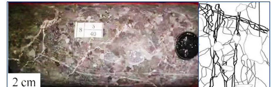
Schematic Diagram of Fractured-Porous Carbonate Reservoir
