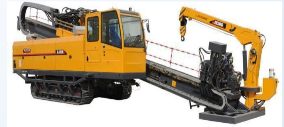
Directional Crossing Drill Rig
